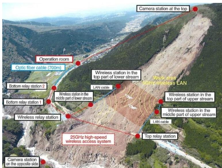
**Fig. 2** A bird's eye view of unmanned construction conducted at Aso bridge district
