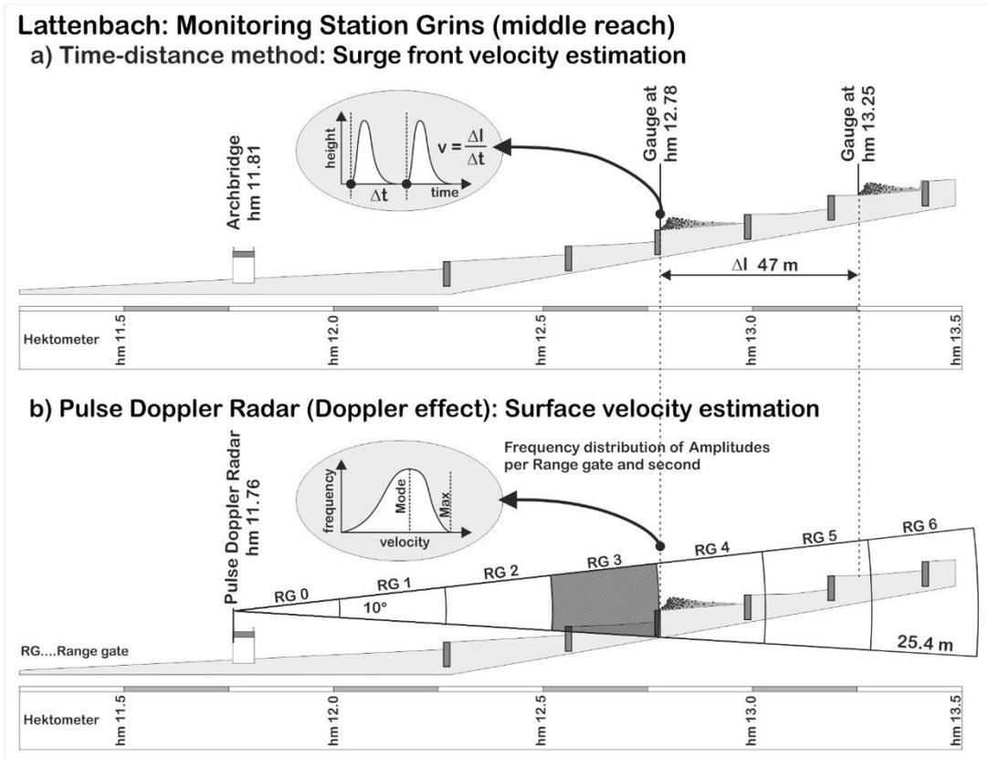
**Fig. 1** Velocity estimation by a) time-distance method and b) application of the Pulse Doppler Radar
