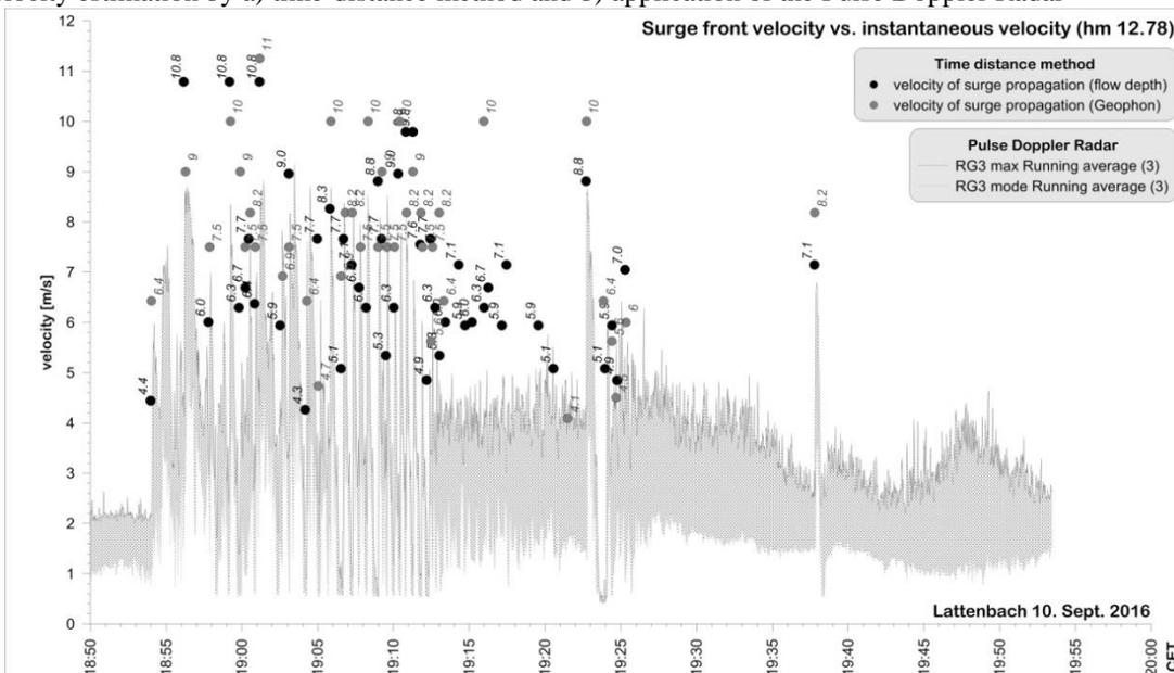
**Fig. 2** Estimated velocities with the different methods for the debris flow on September 16<sup>th</sup>, 2016 at hm 12.78
