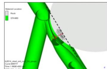
**Fig.4** Local deformation profile at impact point against rock impact
