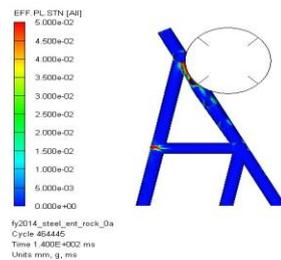
**Fig.3** Damage of steel open dam
