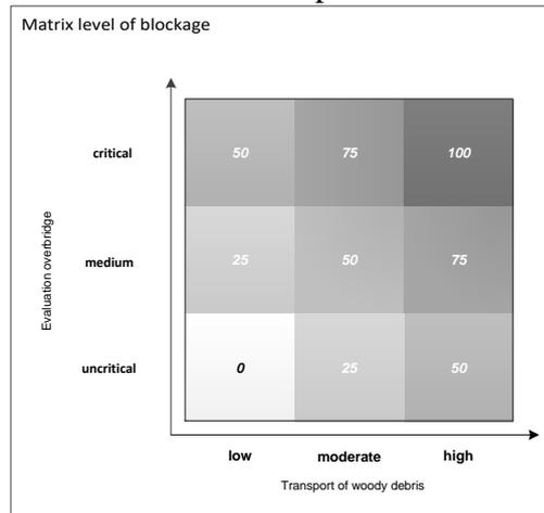
**Fig. 2:** Matrix level of closure for hydraulic 2D-modeling: Combination between *evaluation intersecting structures* (y-axis) and *transport of woody debris* (x-axis).
