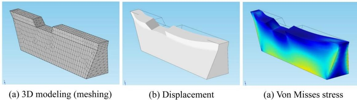
**Fig. 1** Structural analysis of concrete ECD
