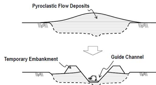
**Fig. 2** Schematic diagram of guide channel
