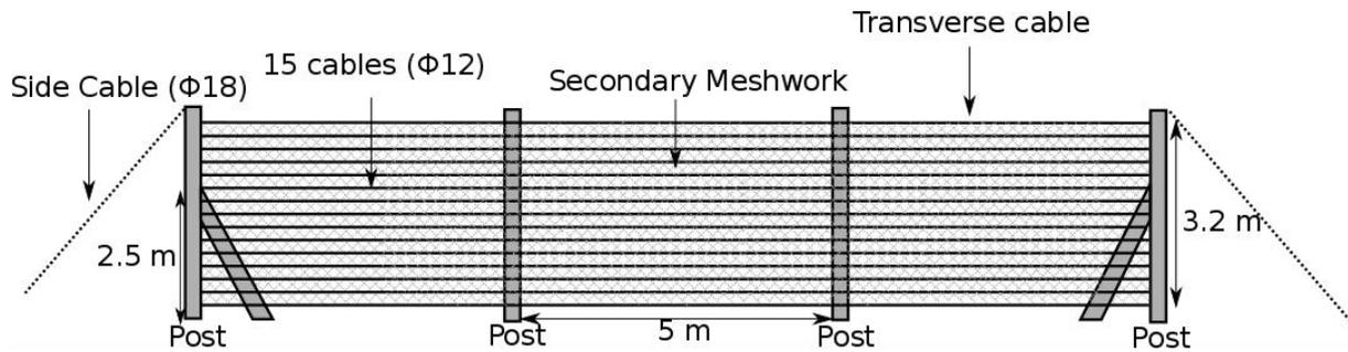
**Fig. 1:** Schematic representation of the barrier.
