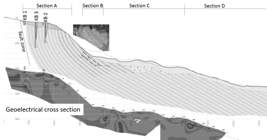
**Fig. 1:** Schematical geotechnical cross section of the landslide with the different sections A, B, C and D.
