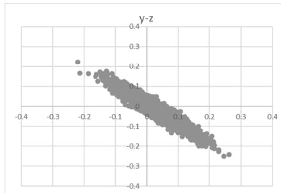
**Fig. 2** Tilt derived from MEMS accelerometer of Y-Z plane
