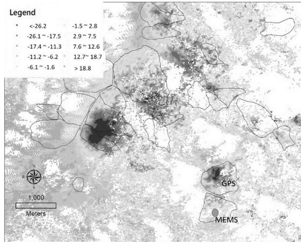
**Fig. 1** Persistent scattering method derived vertical deformation from 2006 to 2016 (unit: mm/year)
