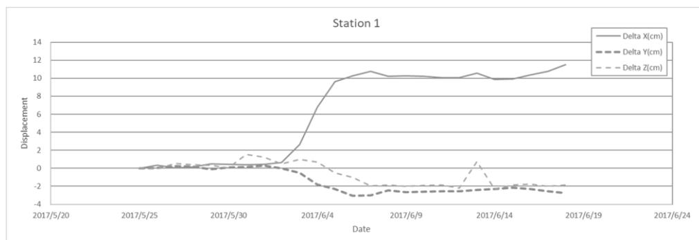
**Fig. 3** GPS monitored result based on rainfall event in June, 2017
