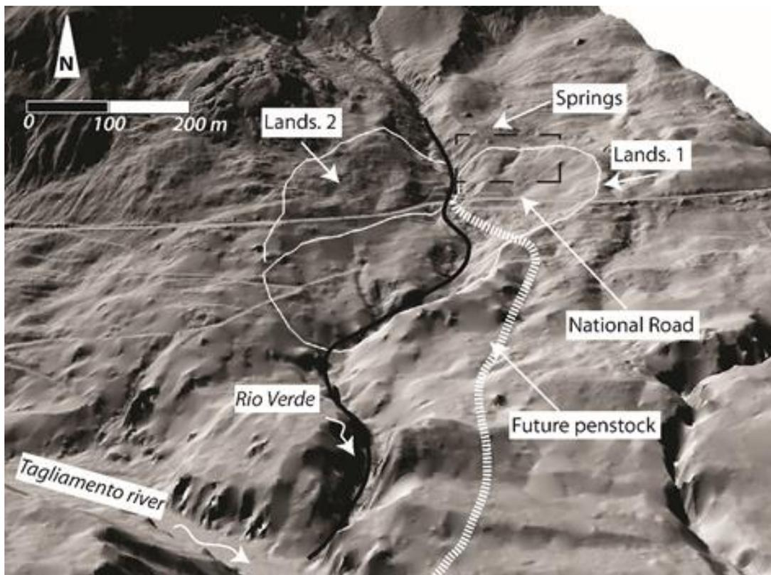
Fig. 2 Study area with possible intervention areas, capitation of water from the springs and buried penstock layout
