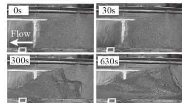
**Fig. 2** Failure process (CASE 1-3)
