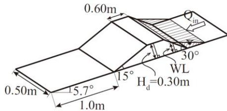
**Fig. 5** Schematic diagram of the flume
