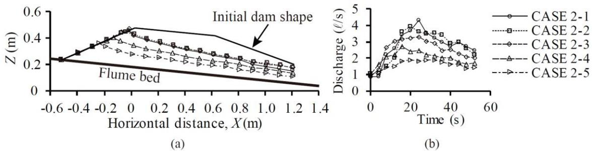
**Fig. 6** (a) Shape of the dam when the reservoir began to overflow and (b) outflow hydrograph.
