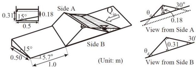
**Fig. 1** Schematic diagram of the flume
