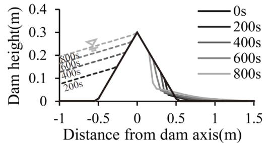
**Fig. 7** Dam deformation process
