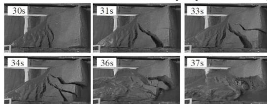
**Fig. 4** Large-scale slip failure (CASE 1-2)
