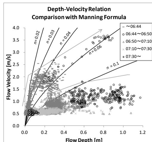
**Fig. 2** Comparison of Depth–Velocity Relation
