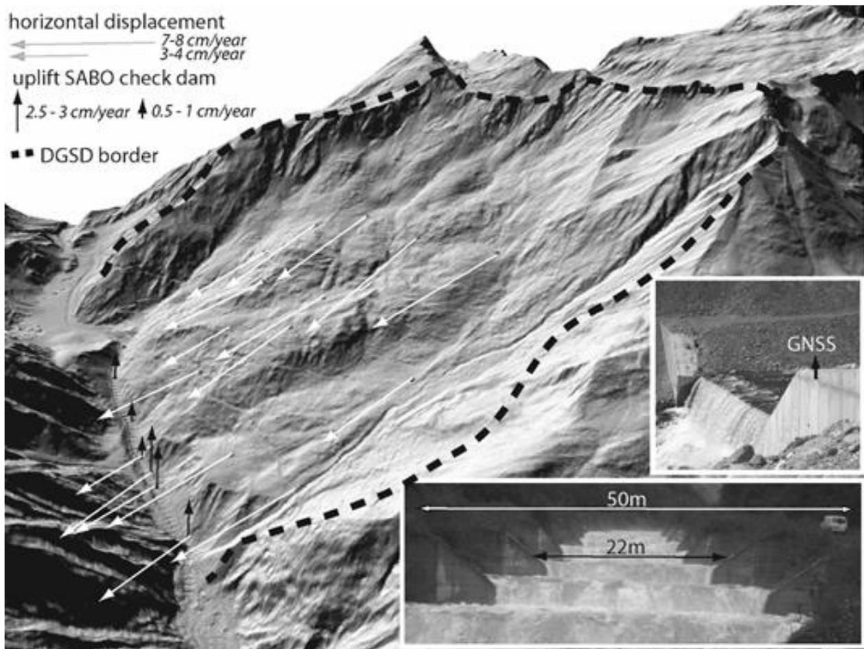
**Fig. 1** GNSS displacements for the benchmarks in the Ganderberg site with two photos of the SABO check dams at the toe of the DGSD
