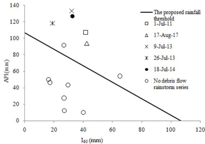
**Fig. 2** The proposed rainfall threshold curve of debris flows in the Guojuanyan gully
