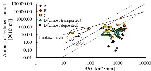
Figure 3. Relationship between sediment transport potential ( $ARI$ ) and sediment runoff.
