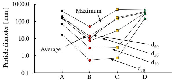
Figure 1. Sediment particle parameters before and after a high-volume sediment production event in the Kawabe River basin.
