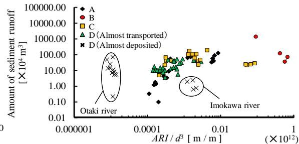
Figure 4. Relationship between sediment transport potential adjusted for particle size ( $ARI / d^3$ ) and sediment runoff.
