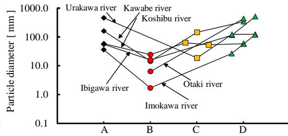
Figure 2. Average sediment particle diameter before and after a high-volume sediment production event.
