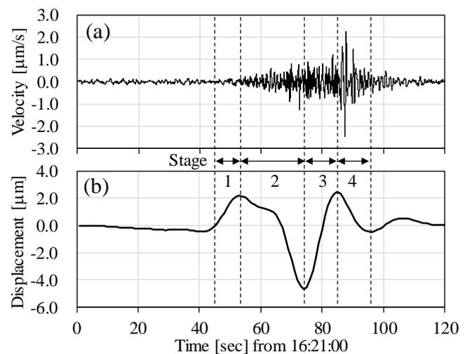
**Fig. 1** Vertical components of (a) 1 – 7 Hz velocity and (b) 0.01 – 0.1 Hz displacement waveforms observed at 35.1 km away from the Akadani landslide in 2011.
