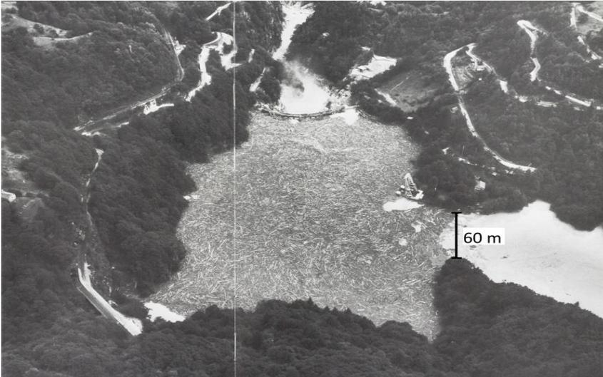
**Fig. 1** Aerial picture of the Palagnedra reservoir after the exceptional August 1978 flood. Approximately 12'500 solid m<sup>3</sup> of LW were deposited upstream of the dam. Source: Heitmann & Zanetti (1980)
