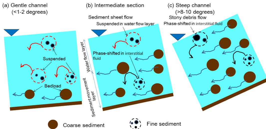
**Fig. 1** Schematic illustration of model
