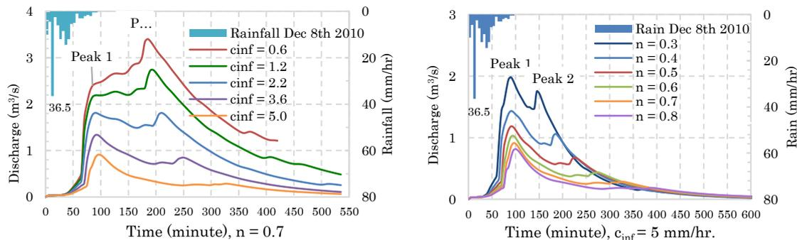
**Fig. 2.** Hydrographs of Manning's,  $n$ , and infiltration coeff.,  $c_{inf}$ , values of Kali Putih
