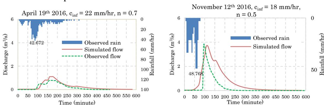
**Fig. 3.** Calibration result for Nasiri River based on April and November 2016 events
