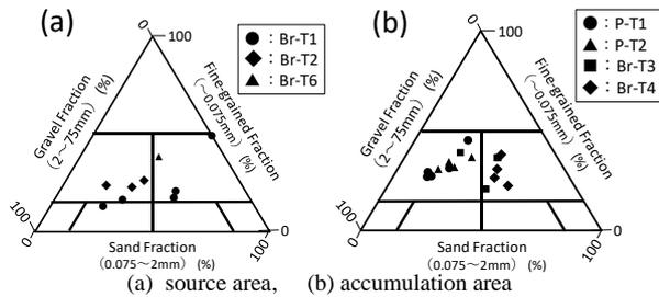
Fig. 1 Grain size distribution of samples from the Tanne-Hirota Landslide
