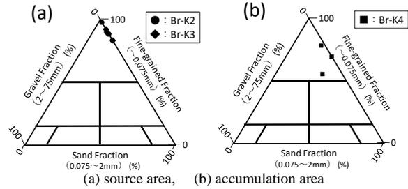
Fig. 2 Grain size distribution of samples from the Kamikozawa Landslide
