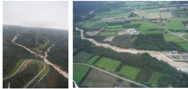
Fig. 2 The sediment discharge in the Pekerebetsu River (Left: debris flow at upper stream, Right: bank erosion and flooding at in the center of Shimizu town, 2016/9/12)
