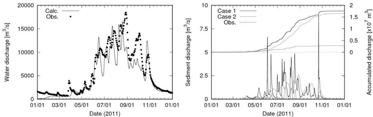
**Fig3** Comparison between calculated and observed value at Sagaing station (left: water discharge; right: uspeded sediment discharge)
