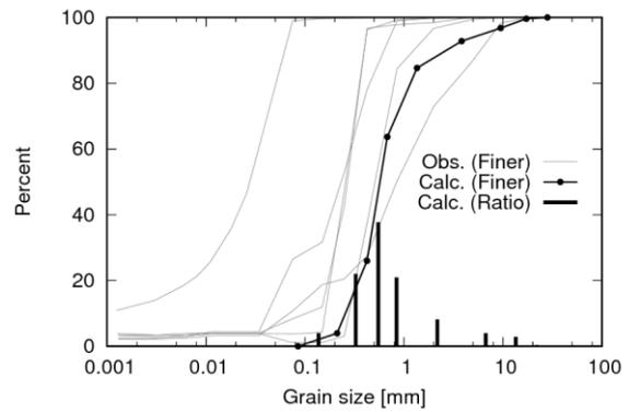
**Fig 2** Grainsize distribution condition of river bed material and produced sediment
