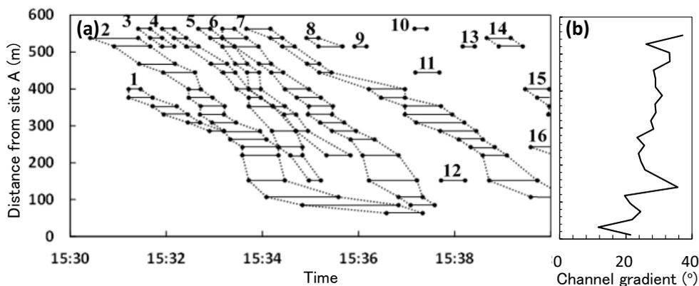
**Fig. 2** Initiation and travel down of debris flow surges in the period from 15:30 to 15:39 on September 10, 2016. (a) Duration of debris flow surges at each analysis points (solid line). (b) Longitudinal profile of channel gradient.
