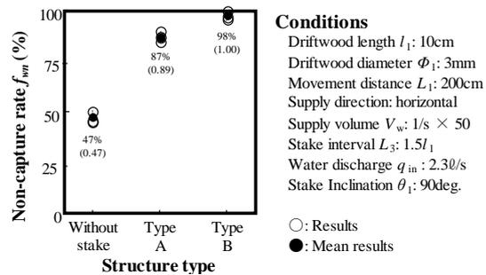
**Fig. 4** Effect of stake type on the non-capture rate\*
