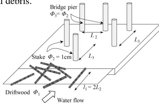
**Fig. 1** Schematic diagram of the experimental setup
