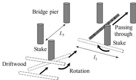
**Fig. 3** Driftwood build-up prevention mechanisms
