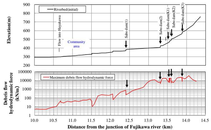
**Fig. 3** Distribution of the debris flow hydrodynamic force along the river in case of haru02
