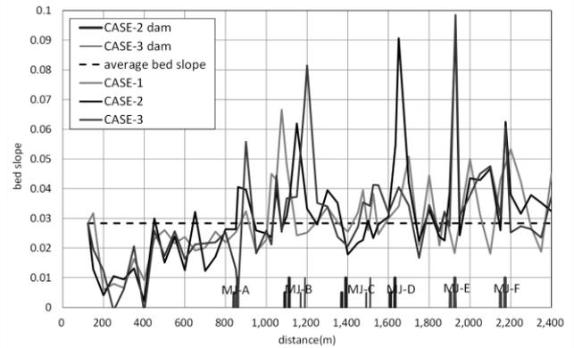
**Fig. 2** Changes in riverbed slope
