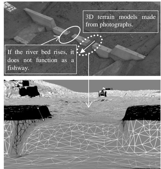
**Fig. 4** Three-dimensional terrain model
