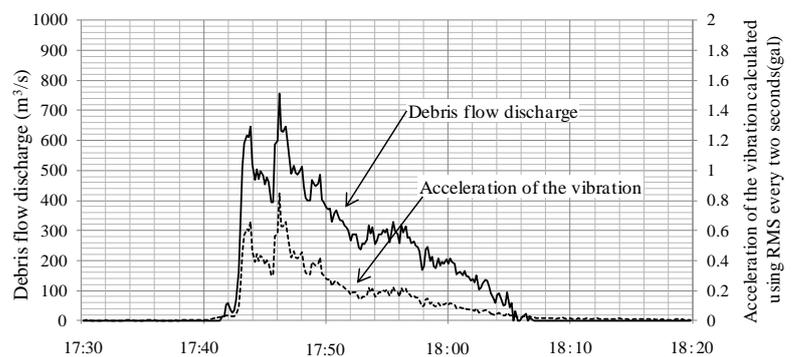
Fig.3 Estimated hydrograph of debris flow
