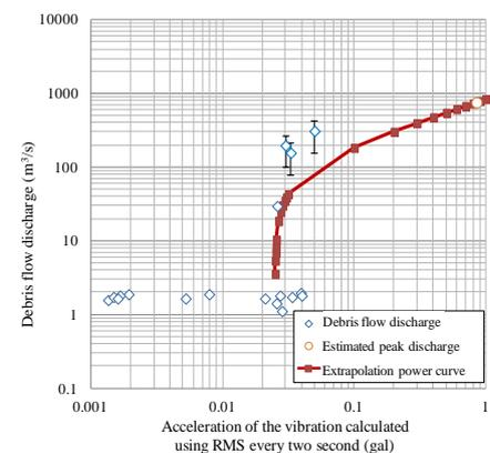
Fig.2 Relations between discharge and acceleration calculated in every two
