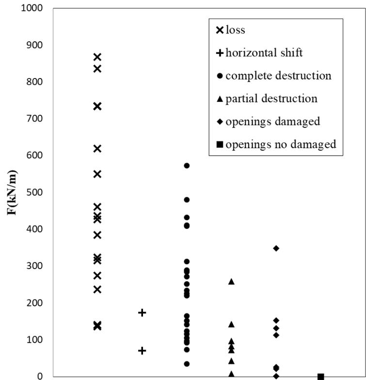
Fig. 1 Distribution of hydrodynamic force(F) categorized by the degrees of damage to wooden residential structures
