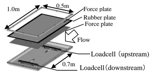
**Fig.1** Schematics of submerged loadcells system
