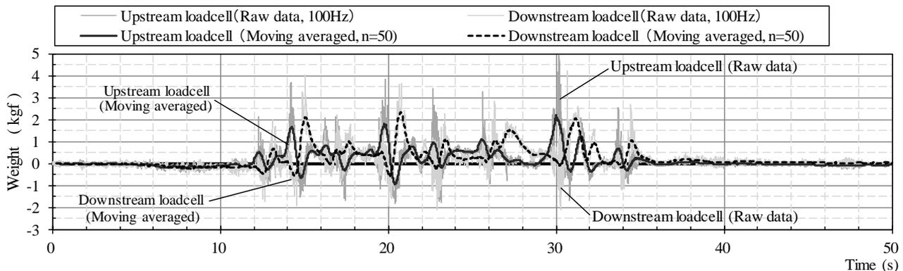
Fig.4 Temporal changes of weight measured by loadcells
