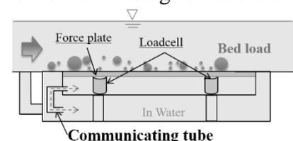
**Fig.3** Schematics of a communicating tube
