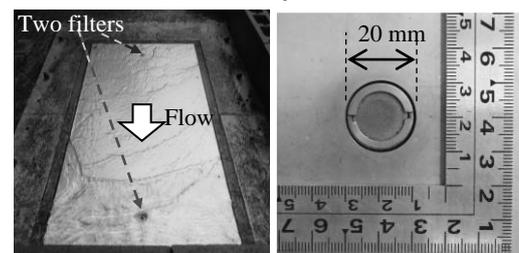
**Fig.2** Two filters on the force plate (Left) and the size of filter in plain view (Right)
